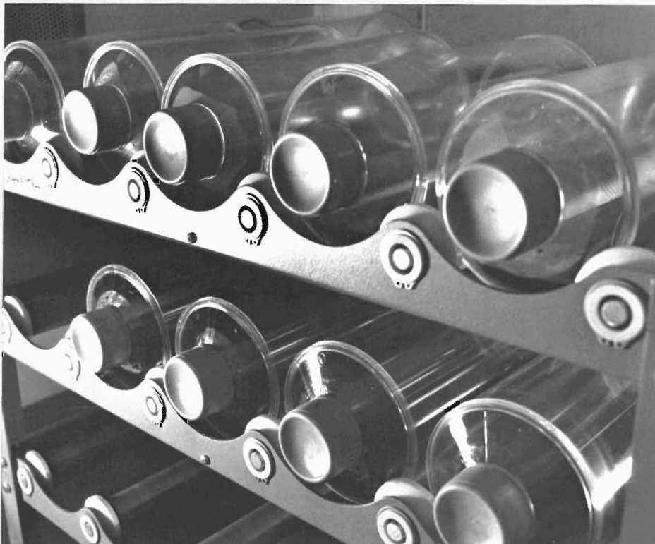
Fig. 2. Cells can multiply manifold in large, slowly rotating cylinders ("roller bottles") since a large surface area is kept in contact with the culture medium.
