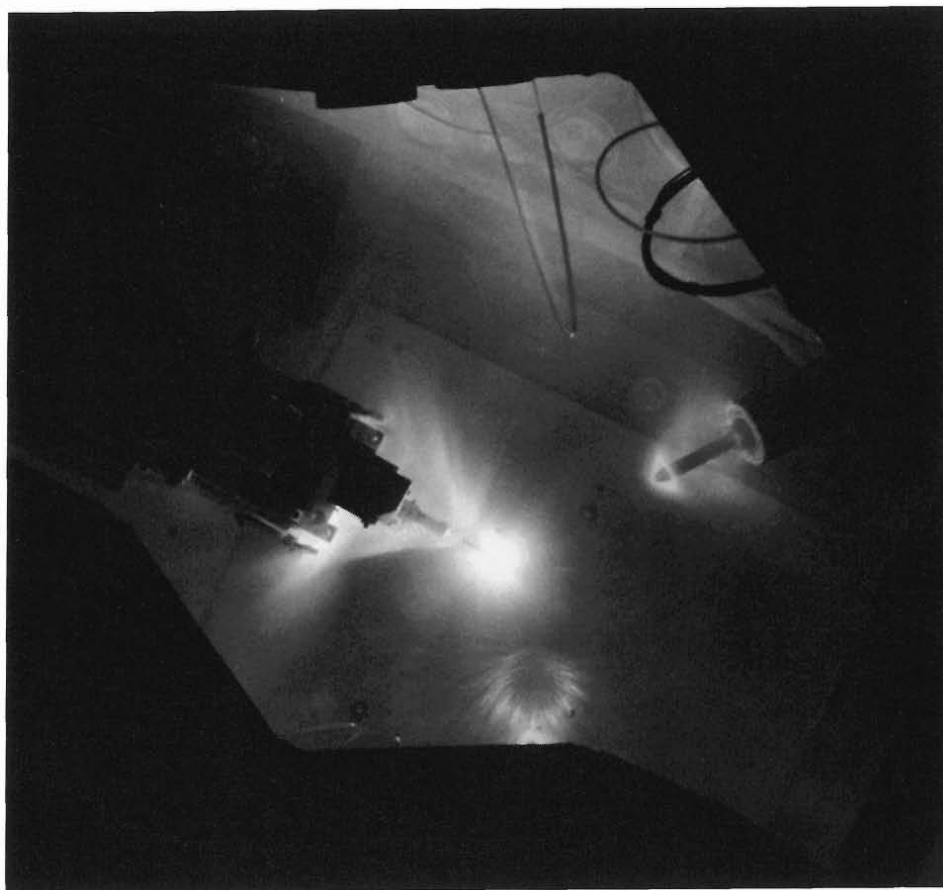
A fusion target bathed in light and plasma during a shot with about 20 kilojoules of energy from Antares. The target is mounted at the end of an insertion mechanism that projects from the left; the object to the right is an x-ray pinhole camera; the circular pattern toward the bottom is a reflection. (Photo by Fred Rick.)
